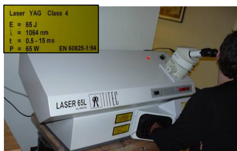
Fig.1: LASER 65 L – TITEC with welding parameters
