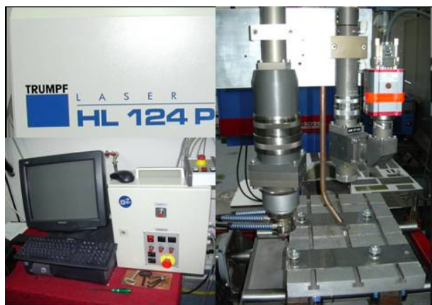
Fig. 1. Laser HL 124P LCU (TRUMPF).
