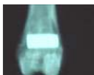
Fig. 1: Apatite-coated porous titanium implants ( \phi 4 \times 10\text{mm} ) with maximal pore size about 240\mu\text{m} . The implants are inserted into the rabbit distal femur.
