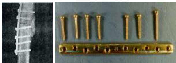
Fig. 1: Plate and screws of AISI 316L
