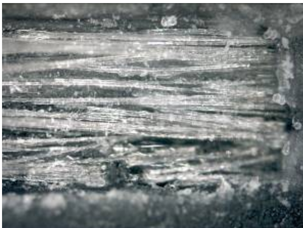
Fig. 1: Retainer side of the fracture zone (50x magnification). The glass fibres lay bare from surrounding EverStick composite/PMMA matrix.
