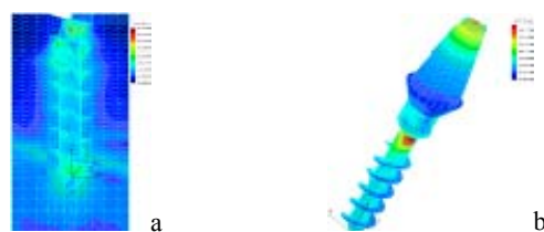
Fig. 3: Von Mises equivalent stress in bone(a) and screw assembly(b)
