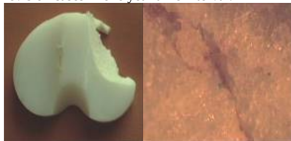
Fig.2: Macroscopic aspects of polyethylene components (left); stereomicroscopic image from failure zone (right)
