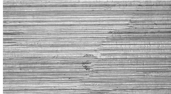
*Fig. 1: Surface finish and roughness in the groove of threads of a TiAl6Nb7 screw processed by thread whirling,  $R_a = 0.2 \mu\text{m}$ .*
