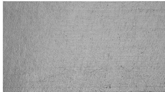
*Fig. 2: Surface finish of the same TiAl6Nb7 screw as in Fig. 1 after rework by CET processing,  $R_a = 0.07 \mu\text{m}$ .*
