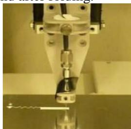
Fig. 1: robotic deposition of UV curable pastes.
