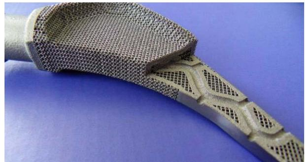
*Fig. 1: Beam Melted hip stem with functional channels and cavities, internal cellular structure and macro-porous surface areas.*
