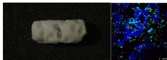
Fig. 1: 12mm Scaffold with 60% (w/w) alginate bead content (left) and (right) seeded with 2 \times 10^5 hMSCs and cultured for 3 days (live = green, dead = red)
