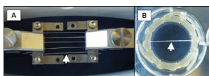
Fig. 1: Experimental set-up for (A) cyclic loading and (B) static conditions. Arrows indicate position of scaffold(s).
