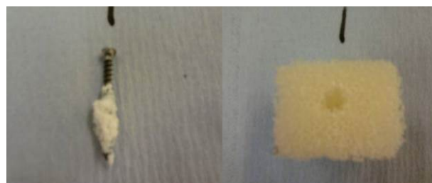
Fig. 2: (left) Screw and attached cement after pullout from sample shown (right).
