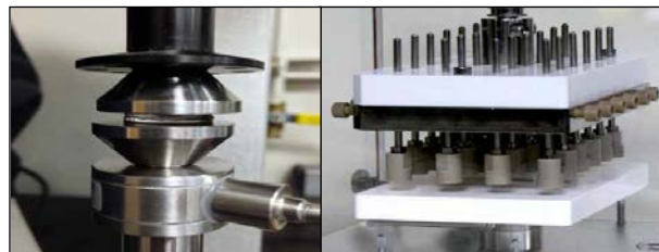
Fig. 1: A single hydrogel specimen was loaded between compression platens for comparison to load data taken on 24 samples simultaneously.
