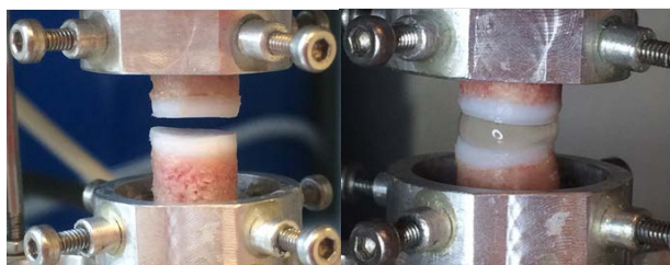
Fig. 1: Schematic representation of the tensile tests performed. The gap in between the osteochondral plugs was first filled with hydrogel before distraction.
