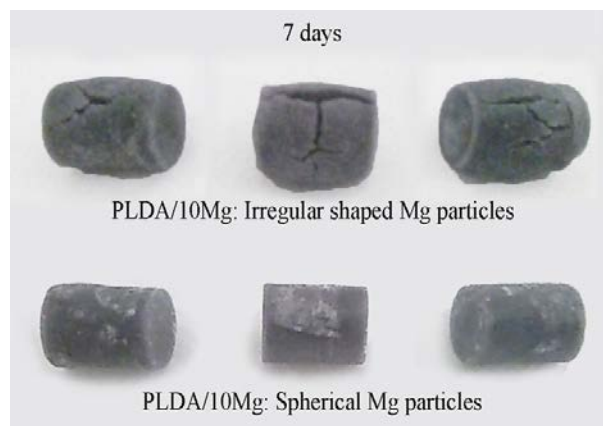
Fig. 1: Photographs of the three specimens of each composite after immersion during 7 days in PBS solution.
