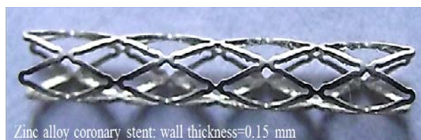
Fig. 1: Zinc alloy made coronary stent with diameter of 2 mm and wall thickness 0.15 mm.
