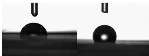
Fig. 2: Wettability of untreated and \text{Al}_2\text{O}_3 -coated PVC samples.
