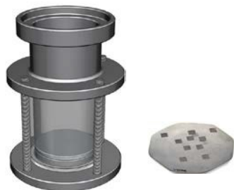
Fig. 1: Safety recipient and building platform (ø65 mm) with selectively melted powder areas.
