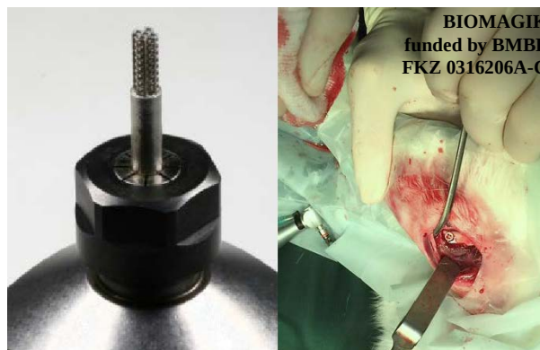
Fig. 1: Magnesium scaffold after fabrication and during insertion in femur for in-vivo testing
