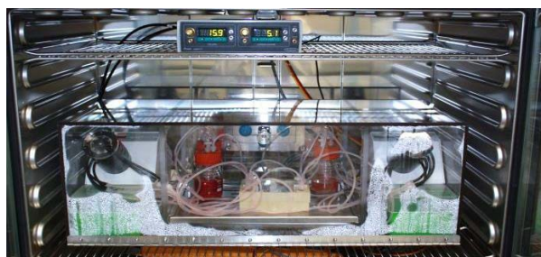
Fig. 1: One of the two dynamic bioreactor setups used within the scope of presented comparative study on degradation of different magnesium alloys
