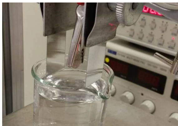
Fig. 1: Experimental set up for electrophoretic deposition. The parameters for Mg alloy substrates have to be carefully adapted.
