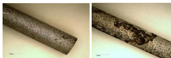
Fig. 2: Mg-0.9Ca: left: sintered and spark-eroded part; right: pitting corrosion after 7 days under cell culture conditions.
