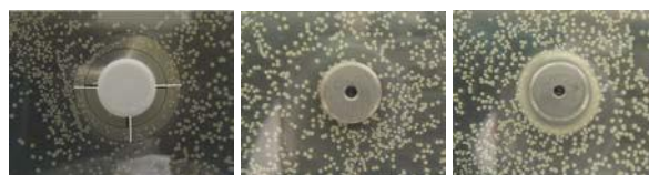
Fig. 2: Growth of S.aureus . a) Standardized \text{Ca}(\text{OH})_2 -loaded tablets are used as positive control: growth is repressed in the inner ring. A diffusion ring extends to the outer ring, b) uncoated Ti as a negative control: No impact to bacteria growth. c) \text{Ca}(\text{OH})_2 -coated Ti: Complete inhibition in the close proximity, reduced bacteria growth in the diffusion zone.
