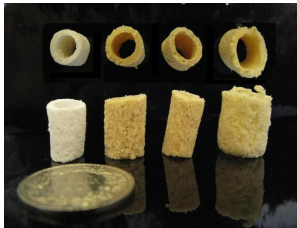
Fig. 1: Image of 3D tubular scaffolds produced from short electrospun nanofibers and shaped via freeze-casting method. From left to right polyamide (PA), pullulan/polyvinyl alcohol (PUL/PVA), polyacrylonitrile (PAN) mixed with PUL/PVA and PAN.
