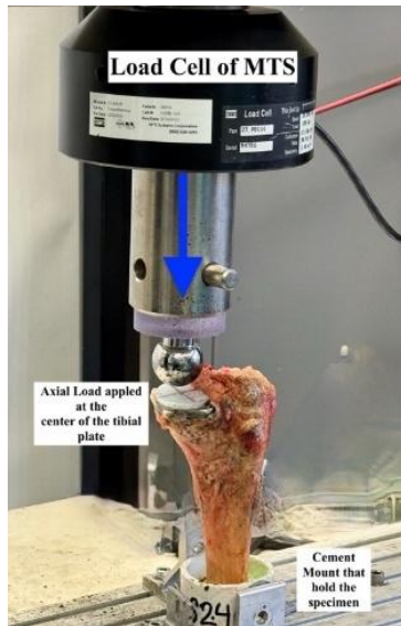
Figure 1: Experimental setup demonstrating the specimen secured in the MTS with axial loads applied (indicated by the blue arrow) until a periprosthetic fracture.
